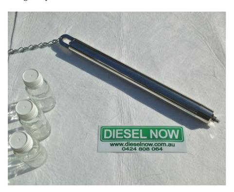
An easy solution is to use a "Bacon Bomb" Sampler to quickly and safely collect Diesel Fuel samples from within 10mm of the bottom of a tank. These Samplers can be inserted through any of the top openings (Fill, Dip, Vent) and they provide a 110 mL sample for evaluation within minutes.
