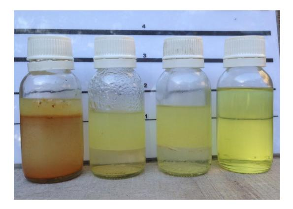
If there is any cloudiness, discoloration, layers, or suspended matter the sample should be sent to an independent Analytical Laboratory for further analyses.
